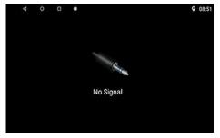
Owhen the car engine is not connected with the equipment, in CAMERA screen shows no signal.
